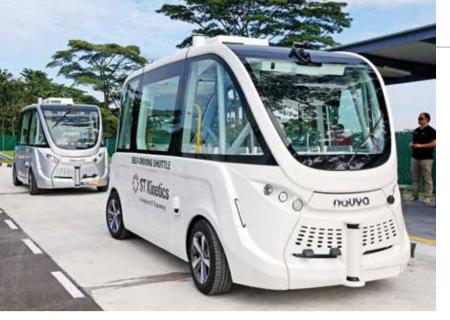
Navya self-driving shuttle bus at the CETRAN Autonomous Vehicle Test Centre. ST PHOTO: GAVIN FOO
